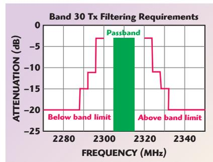
▲ Fig. 4 Band 30 uplink filter requirements.
